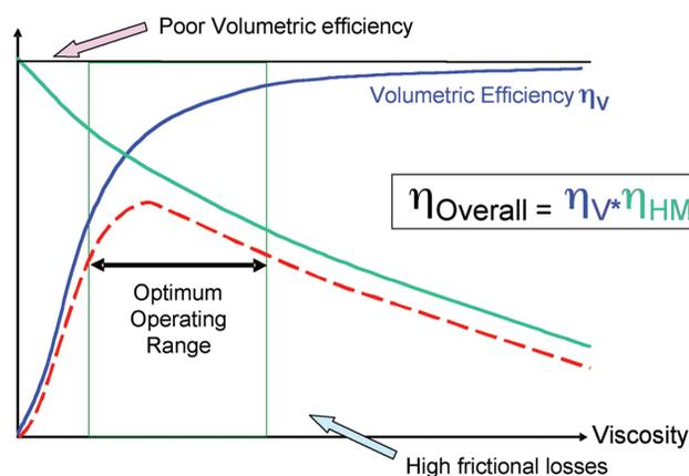
The most effective hydraulic fluids are thin enough to allow the most efficient flow, and thick enough to pump with the greatest efficiency. Viscosity changes with temperature, so an efficient hydraulic fluid must maintain optimal performance at a wide range of temperatures, from cold equipment start-up to the heat that builds up during extended periods of operation.<sup>4</sup>
