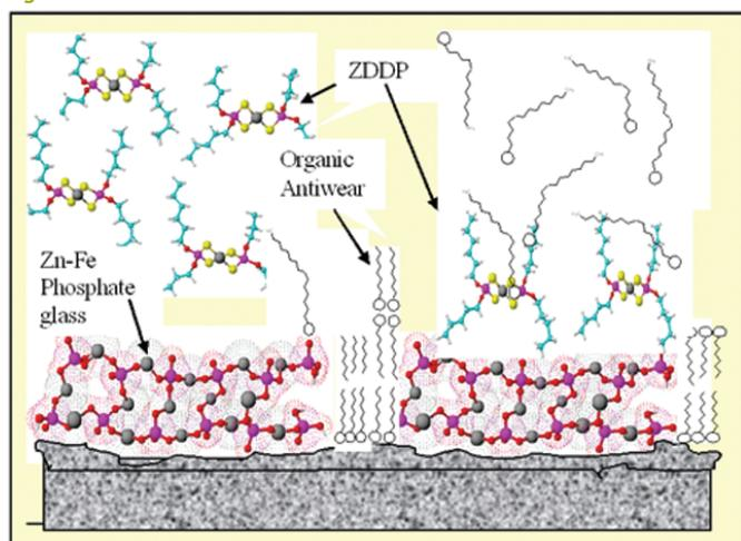
Schematic representation of the development of Zinc-Iron - polyphosphate films derived from the decomposition of ZDDP at extreme pressure and temperature in the boundary layer lubrication conditions near the piston ring cylinder contact surface.
