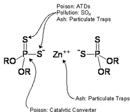
The molecular structure of ZDDP, indicating the elements of detrimental to both the performance of environmental pollution control devices and contributing to SOx, and particulates.
