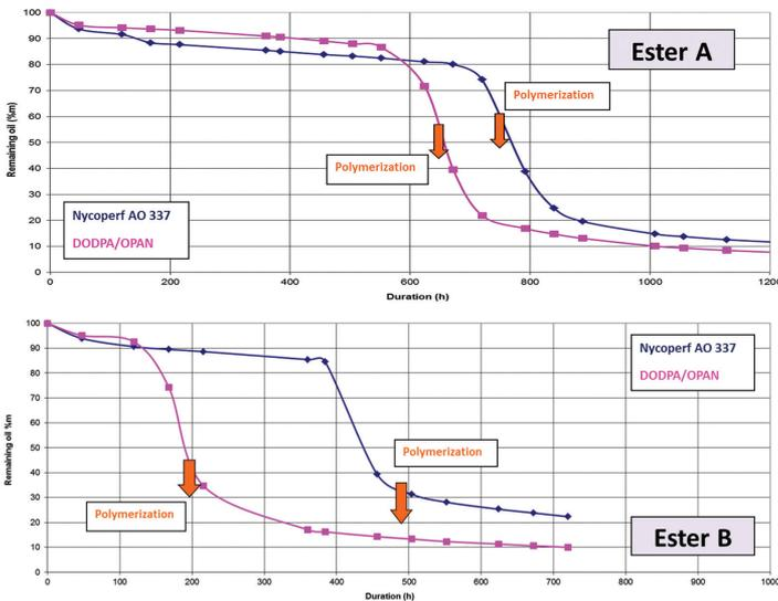
Figure 3. Pan test, evaporation graphs, 200°C.
