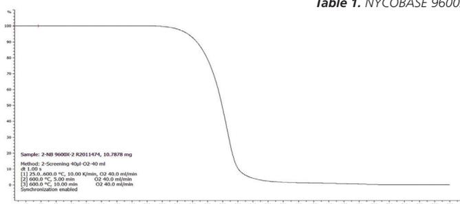
Figure 2. NYCOBASE 9600X - Thermogravimetry (dynamic)
