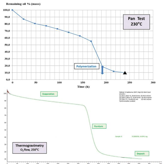
Figure 4. Pan test at 230°C and thermogravimetry of NYCOBASE 9600X with NYCOPERF AO337.
