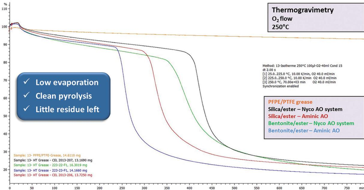
Figure 5. Thermogravimetric analysis, 250°C
