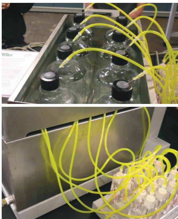
Figure 3: 301 F biodegradability test instrument: (above showing the sample test bottles in water bath with cover removed); and (below) Oxygen flowmeters feeding oxygens to the test bottles.
