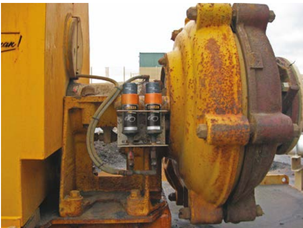
Figure 1: Single-point lubricators periodically deliver grease or oil to bearings, chains and other industrial equipment components.
