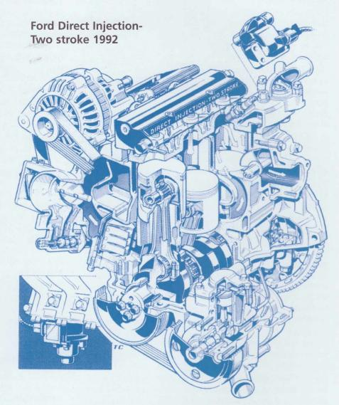
With twice as many firing pulses per revolution, a three-cylinder 2T's running refinement is similar to that of a six-cylinder 4T. Its faster response also gives it an enhanced performance feel.
