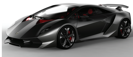
Figure 2 Engineering marvel or an exercise in extreme weight loss? Lamborghini Sesto Elemento super sport car has a body constructed of CFRP, resulting in a curb weight of just 999 kg for the vehicle powered by 562 hp V10 engine and permanent all-wheel drive (Photo courtesy Autoguide.com).
