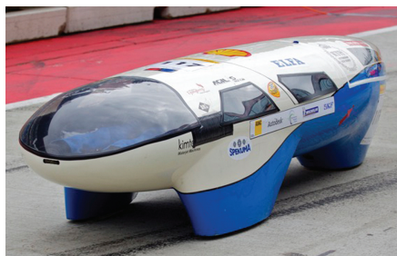
Figure 1 Is that what the car of the future will look like? Agelis ecocar built at Royal Institute of Technology, KTH, Stockholm, Sweden, managed to run for 481 km at 1 L of gasoline during Shell Eco Marathon 2010. Critical engine components had antifriction coatings made by Applied Nano Surfaces and a fuel-economy engine oil produced by Elektrion s.a. was used.
