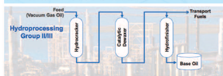
Group II/III: All-hydroprocessing Conversion used better than extraction
