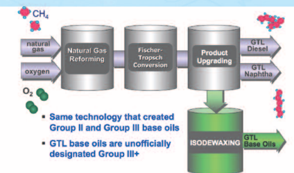
ISODEWAXING (Hydroisomerization) technology enables GTL base oils
