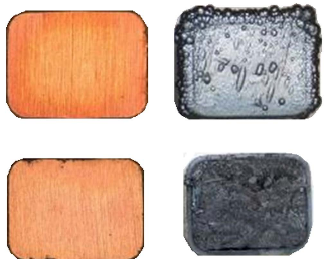
Figure 3: Results from copper corrosion test run at 150°C in closed vessel, to the left an eFluid, to the right the same eFluid but with 10% axle oil added to it. On top row from the part or the piece exposed to the vapour phase and the bottom row exposed to the oil phase
