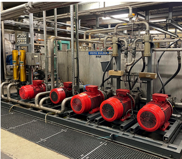
Figure 11: Hydraulic system for cooling and bearing lubrication as part of the Nipco-Roll.
