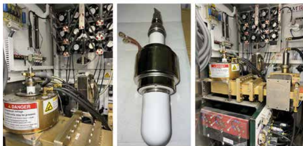
Figure 11: Industrial Magnetron (915MHz) as Installed within the Transmitter 12
