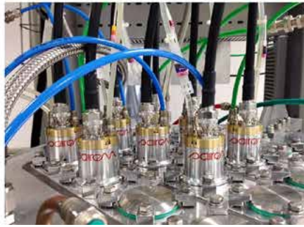
Figure 7: Ann ECR coaxial microwave plasma source that can be used in arrays for application to larger surfaces 8
