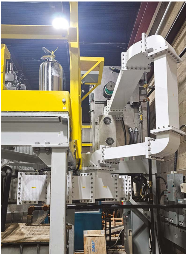
Figure 1: Microwave-operated kettle used for manufacturing grease, Source Patterson Industries Canada.
