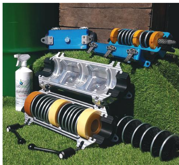
Figure 6: A dual chamber clam shell type wire rope lubricator Courtesy of Lubitec UK
