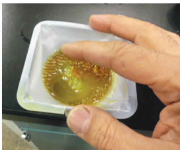
Figure 3: Vegetable oil exposed to heat and air forming a layer of polymer Source: Environmental Lubricants Manufacturing, Inc.
