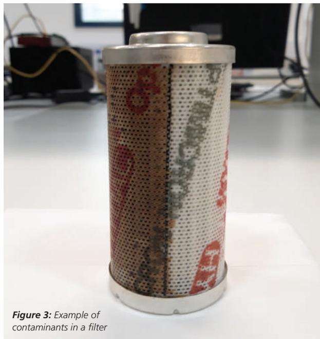
Figure 3: Example of contaminants in a filter
