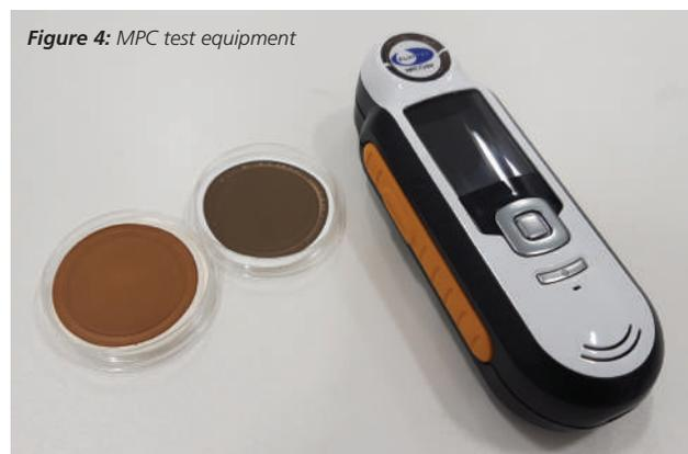
The MPC (Membrane Patch Colourimetry) Test – traditionally developed for turbine lube oil applications, this procedure extracts any insoluble contaminants onto a filter membrane and assigns an index value based on colour; essentially, the darker the membrane, the greater the risk of varnish deposition in the system. The number scale is typically interpreted as follows:
