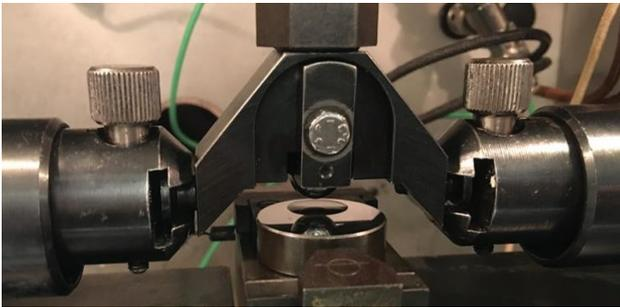
**Picture 1:** Shows the oil sample between the Disc and Ball in SRV-rig.
