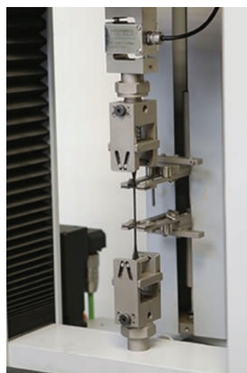
Figure 5. Traction machine used for seal tensile strength and elongation at break
