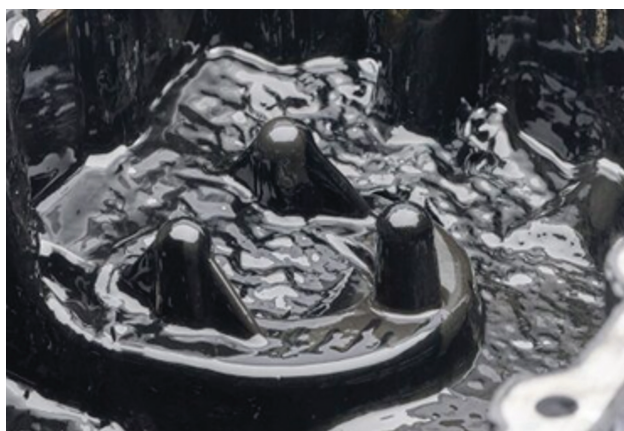
Figure 5: Illustrates the oil sump condition following engine testing at Lubrizol's test facility. The top image displays the results with OEM-approved engine oil, while the bottom image shows the results with a SFU engine oil. This image is owned and protected by Lubrizol.
