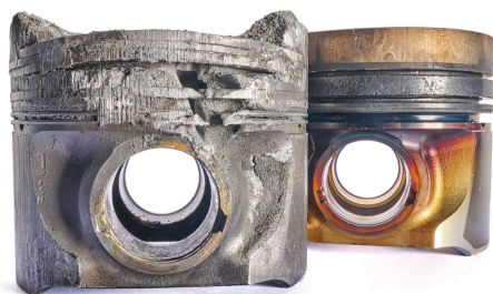
Figure 1: Is engine oil testing and OEM approval necessary? The image illustrates a comparison between pistons from an engine test conducted at Lubrizol's test facility. The piston on the left was tested with an SFU engine oil, which failed at 23 hours, while the piston on the right used an OEM-approved engine oil, successfully completing the full test at 96 hours. This image is owned and protected by Lubrizol.
