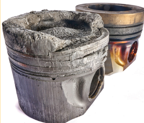
Figure 6: The image illustrates a comparison between pistons from an engine testing conducted at Lubrizol's test facility. The front piston is from an engine tested with a SFU engine oil, which failed at 23 hours, while the rear piston is from an engine using an OEM-approved engine oil, successfully completing the full test at 96 hours. Image owned and protected by Lubrizol.
